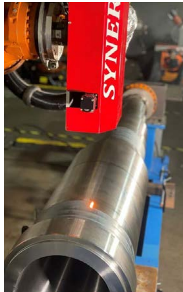
Figure 5. Laser heat treating the OD of large industrial shaft used in paper mills
