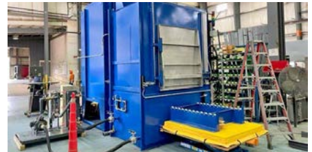
New, fully automated quenching system
