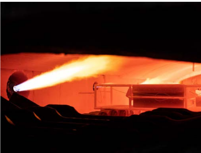
Figures 3. Temperature uniformity survey of a continuous furnace using the plane method applying the PhoenixTM thru-process monitoring system. The data logger travels protected in a thermal barrier mounted on the TUS frame performing a safe TUS at four points across the width, which is impossible with trailing thermocouples. (Source: Raba Axle, Győr, Hungary)
