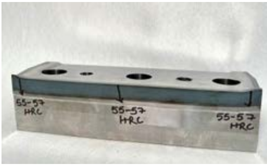
Figure 3. Laser heat treated trim inserts (approximate dimensions of 7" x 4" x 3", base material 4140) demonstrate distortion of less than 10 microns and hardness of 55–57 HRC.
