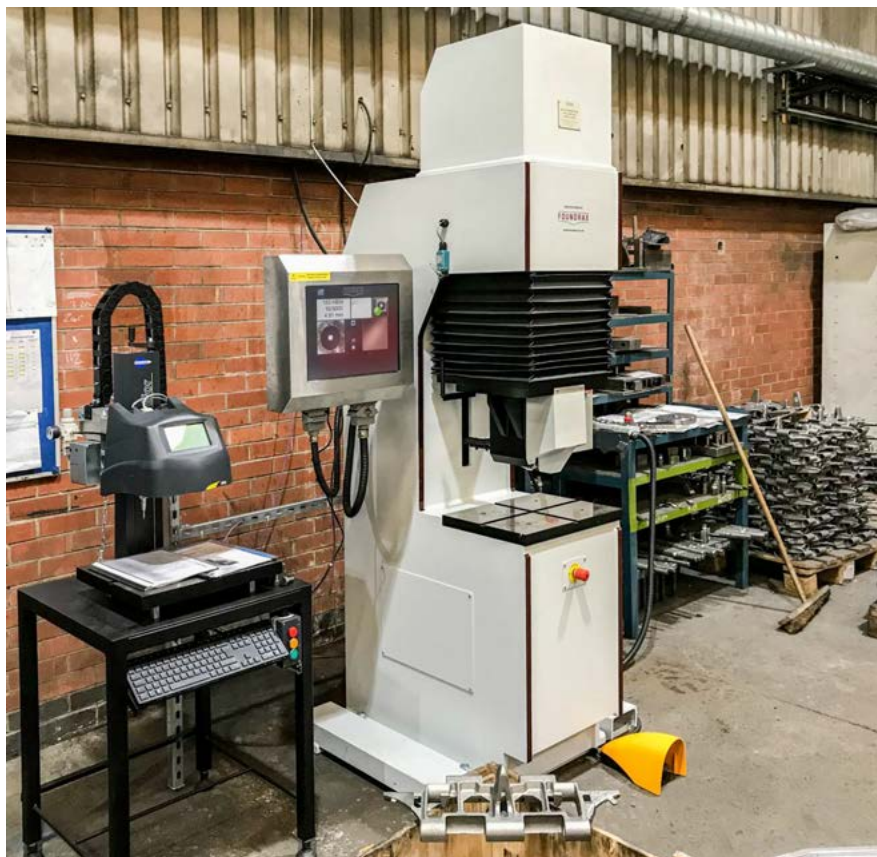
Figure 1. Heavy-duty Brinell tester in situ Figura 1. Robusto probador Brinell in situ
