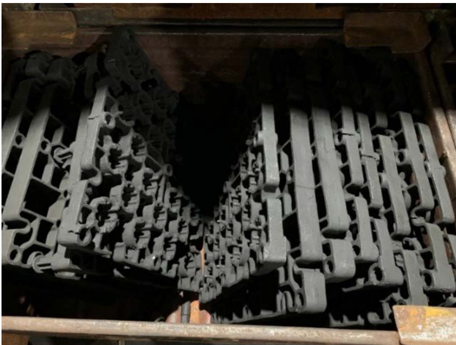
Figure 7. Typical scrap alloy trays and grids (Source: Castalloy Group)
