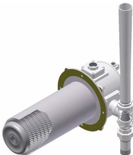
Direct fired self-recuperative burner
