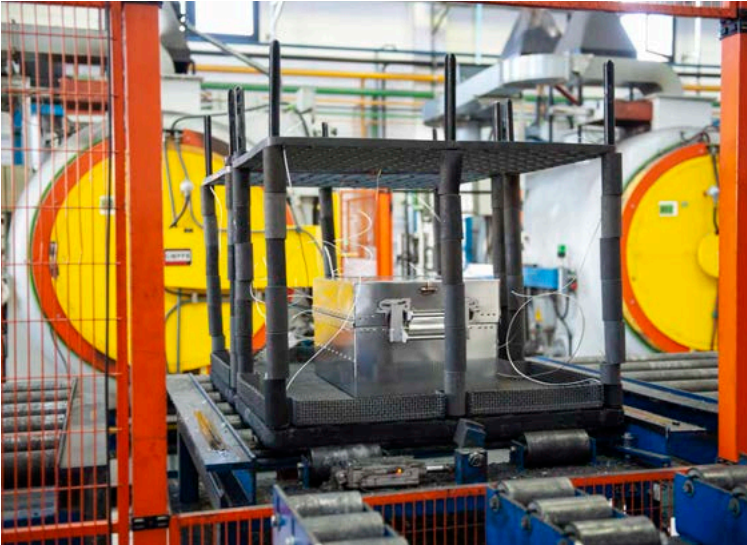
Figures 5. (left) Thermal barrier being loaded into LPC batch furnace with TUS frame as part of temperature uniformity survey. (right) Thermal barrier shown with independent quench deflector providing protection during the high pressure gas quench. (Source: Phoenix™)
