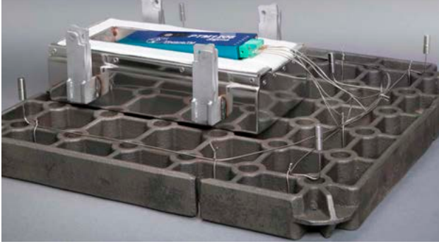
Figure 6. (left) Low profile TUS system (TS02-128-1 thermal barrier six channel Sigma data logger) designed with TUS surveying individual one-piece flow heat treatment LPC furnace chambers. (right) Thermal barrier shown with optional low profile gas quench deflector. (Source: PhoenixTM)
