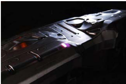
Figure 1. Laser heat treating performed on Class A die
