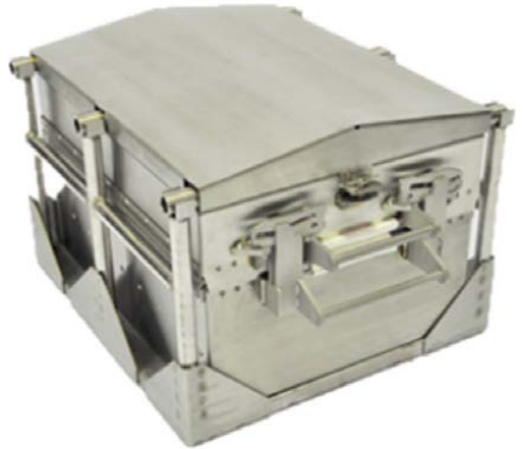
Figures 5. (left) Thermal barrier being loaded into LPC batch furnace with TUS frame as part of temperature uniformity survey. (right) Thermal barrier shown with independent quench deflector providing protection during the high pressure gas quench. (Source: Phoenix™)
