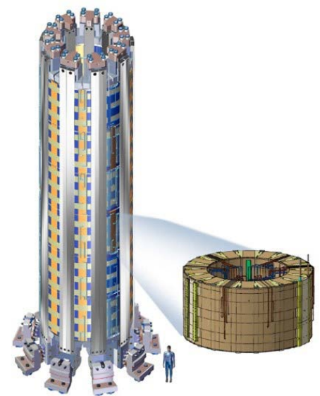
Figure 2. ITER central solenoid and one isolated solenoid module
