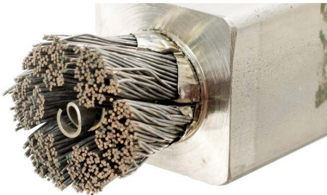
Figure 3. A dissection of the central solenoid conductor strands, central spiral, and structural jacket
