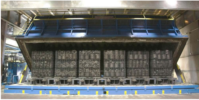
Indirect gas-fired atmosphere furnace used to handle a variety of parts. Work chamber is approximately 31' x 9' x 9' and has a load capacity of 90,000 lbs. Source: Premier Furnace Specialists
