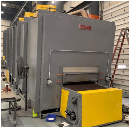
Continuous conveyor furnace for firearm manufacturer
