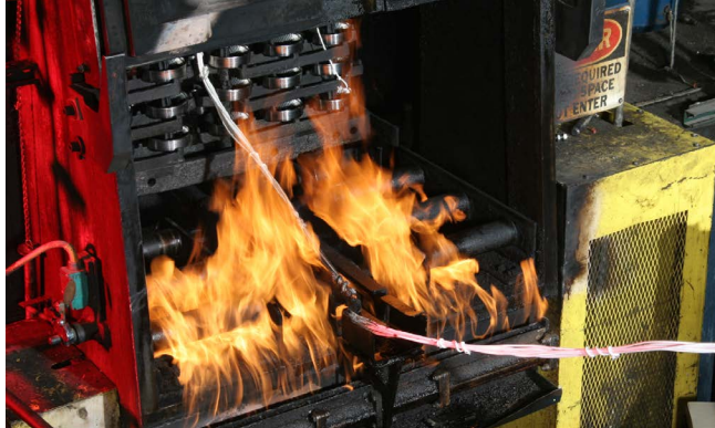
Figure 1: TUS using type K expendable thermocouple insulated in ceramic fiber
