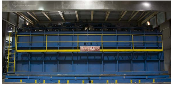
Indirect gas-fired atmosphere furnace used to handle a variety of parts. Work chamber is approximately 31' x 9' x 9' and has a load capacity of 90,000 lbs. Source: Premier Furnace Specialists
