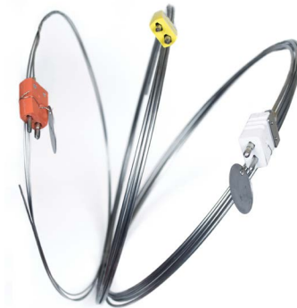
Figure 2: Non-expendable type N and K mineral insulated thermocouples
