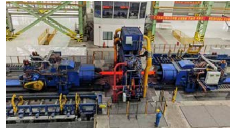
Hydraulic radial forging line for aerospace materials
