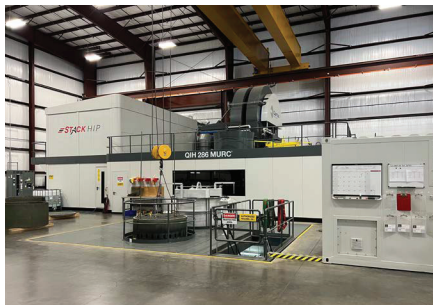
Stack HIP equipment (Source: Stack Metallurgical Group)
