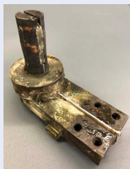
Soap and hot water will remove sticky quench and debris. (Source: Induction Tooling, Inc.)
