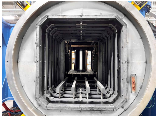
Hot zone (Source: Solar Manufacturing)
