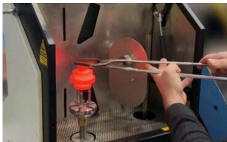
"The hot forged parts are picked up as they leave the press and directly placed into the measuring cell." (Source: nokra)
