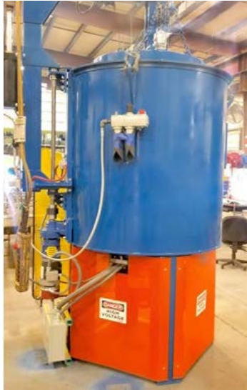
Steam atmosphere pit furnace
