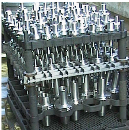
Figure 4a and 4b. From left to right: CFC level grid (case hardening, oil quench); CFC-Rack CVD-Coating
