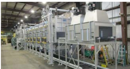
New roller hearth system
