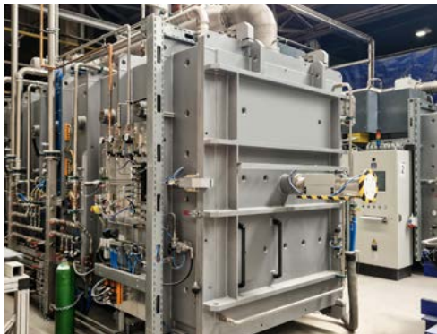
At the RATH plant in Krummnußbaum, Lower Austria, two new vacuum nitriding furnaces are being operated. (Source: heat processing)
